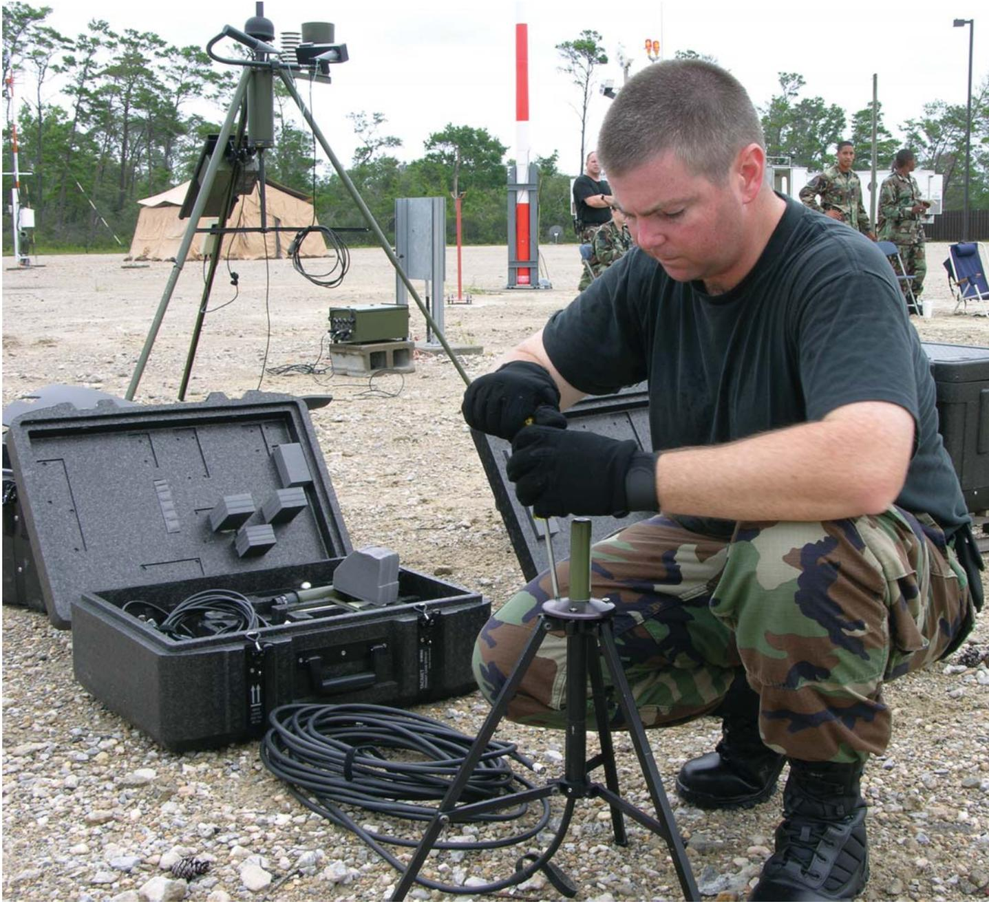
Technical Sgt. Todd Von Almen, a weather operations analyst at the Air Force Combat Weather Center, Hurlburt Field, Fla., attaches an Iridium antenna to a tripod for use with the A/N TMQ-53 Tactical Meteorological Observing System. The weather sensor is used by deployed units to gather weather observations in support of base operations and local flying missions. Photo courtesy of the Air Force Combat Weather Center.
