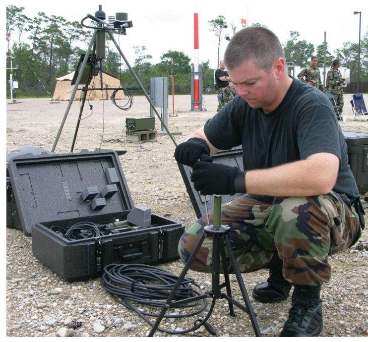
Technical Sgt. Todd Von Almen, a weather operations analyst at the Air Force Combat Weather Center, Hurlburt Field, Fla., attaches an Iridium antenna to a tripod for use with the A/N TMQ-53 Tactical Meteorological Observing System. The weather sensor is used by deployed units to gather weather observations in support of base operations and local flying missions. Photo courtesy of the Air Force Combat Weather Center.
