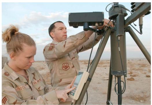
Senior Airman Laci Wood collects weather data from a TMQ-53 while Tech. Sgt. Carlton Hatfield readjusts the system's transmitter. It is one of several methods the 455th Air Expeditionary Wing's combat weather team at Bagram AB, uses to gather detailed weather updates hourly for pilots and Combined Joint Task Force 76 operations planners. Airman Wood is deployed from Eglin AFB, Fla., and Sergeant Hatfield is from Shaw AFB, S.C. Photo by Staff Sgt. Jennifer Lindsey.
