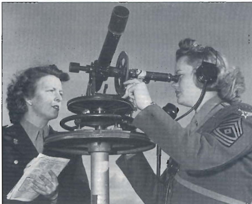
Photo from former Army Air Force Training Command, HQ AAF Western Flying Training Command, Santa Ana, Calif. Sergeant Christina L. Meaner (right) follows the movements of a pilot balloon with the theodolite, as Lt. C.J. Nolan checks the reports.
