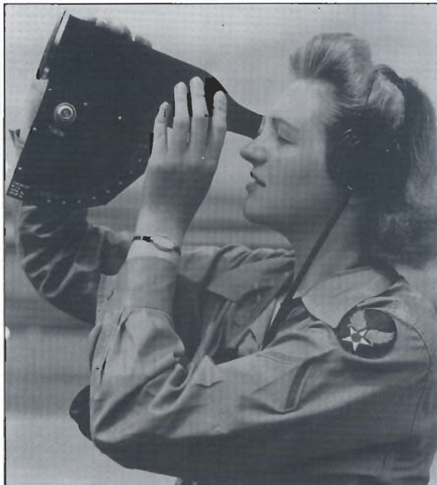
Photo from AAFTF, HQ AAFFWTC WAC Private 1st Class Angela Michael uses a clinometer to test cloud ceiling at Carlsbad Army Air Base, N.M.
