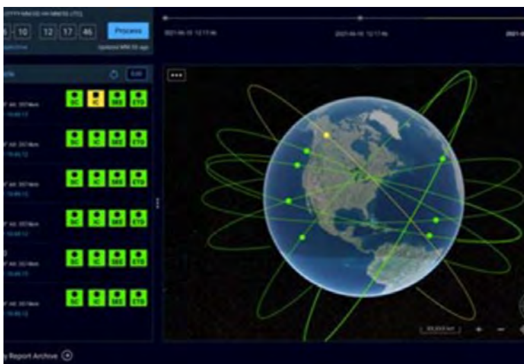
Energetic Charged Particle - Hazard Assessment System (ECP-HAS) tool. Designed to provide satellite drivers, space operations centers, and environmental providers a single application that can evaluate environment effects to spacecraft in any orbit
