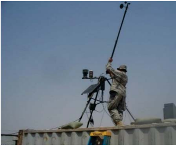
Assembling a TMQ-53 Tactical Meteorological Observing System.
